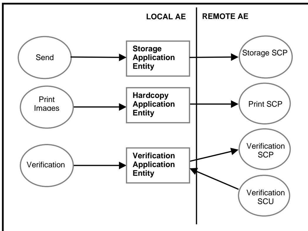
– The Storage Application Entity sends images to a remote AE. Sending images depends on user configuration, “Batch”, “Send As You Go” or “Manual”. For “Batch” and “Manual” configuration, the system opens an
